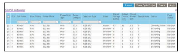
The delivered power is stated in the Output Power (W) column (4.6W for Port 1 in the previous figure).
