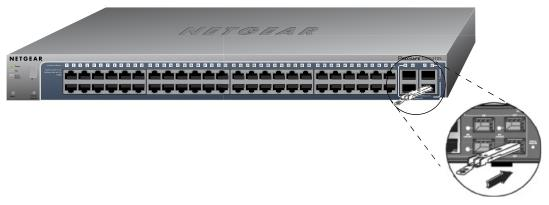
Figure 9. Installing an SFP transceiver module
