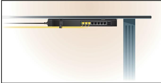
**Figure 9. Strap the cables to the bracket**
