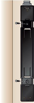
Note: You must screw the backplate into a wall stud.
