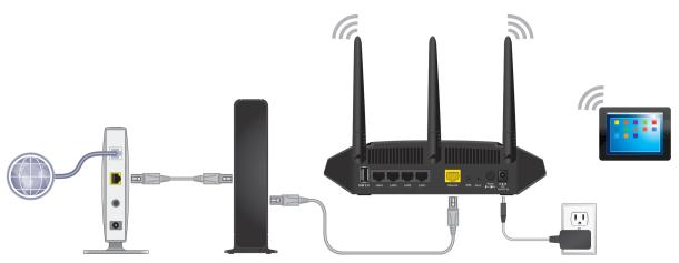
Figure 4. Connect the access point/router to another router in your network
