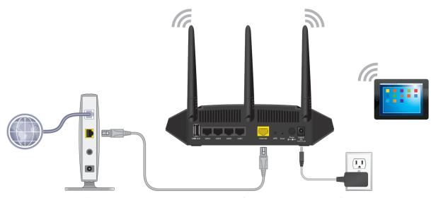
Figure 5. Connect the access point/router in router mode to your Internet modem
