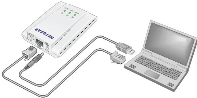
Figure 5. Connecting the wireless access point to a laptop
