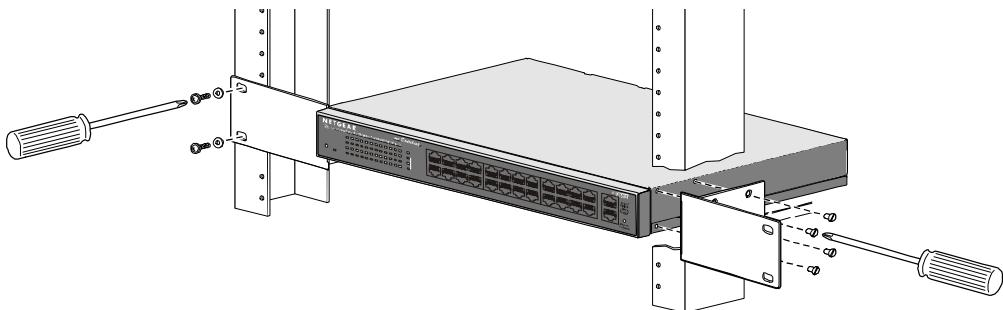
**Figure 4-1. Attaching Mounting Brackets**
