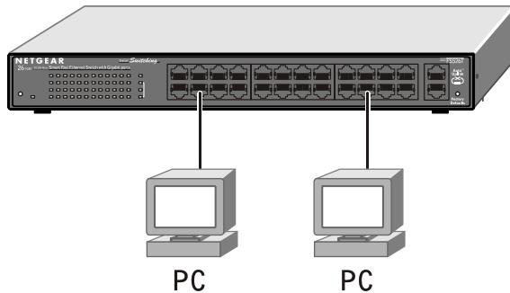
**Figure 4-4. Connecting Devices to the Switch**
