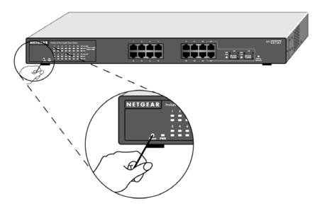
Figure 2-3. Reset Button of the GS716T Gigabit Smart Switch
