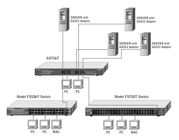
Figure 3-2. Example of Backbone Switching
