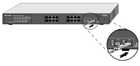
Figure 4-3. Installing a SFP GBIC Module into GS716T
