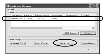
The Smartwizard Discovery utility finds the switch and displays its MAC Address, IP Address, and model number. If you cannot configure your switch, verify that the cable connections are secure, that the IP address configuration of the PC is in the same subnet as the switch, and click the Discover button.
