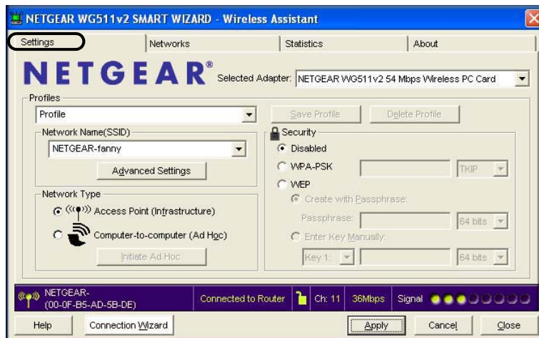
Figure 3-2: Access Point (Infrastructure) mode
