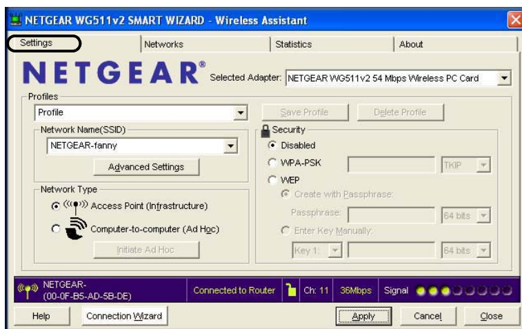
Figure 3-4: Computer to Computer (Ad Hoc) mode
